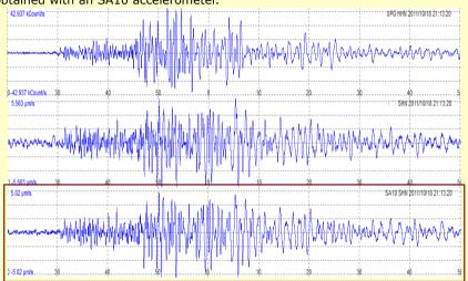
You can notice that, being P and S waves of same amplitude, the background noise of the first 10 seconds is much lower in the SA10 and also more clean in the respect of the competitor.
